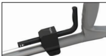
**Note:** Check that the twist lock on the handle of the STEETS Steady Stand is open as this is the only way to pull the upper subsystem upwards.
